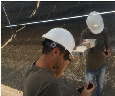
*Picture: Measurement of soiling and cleanliness at parabolic trough solar mirror with pFlex mobile device*
